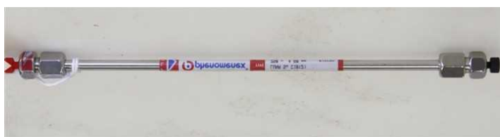
Figura 18. Columna Phenomenex Luna 00G-4252-E0.
