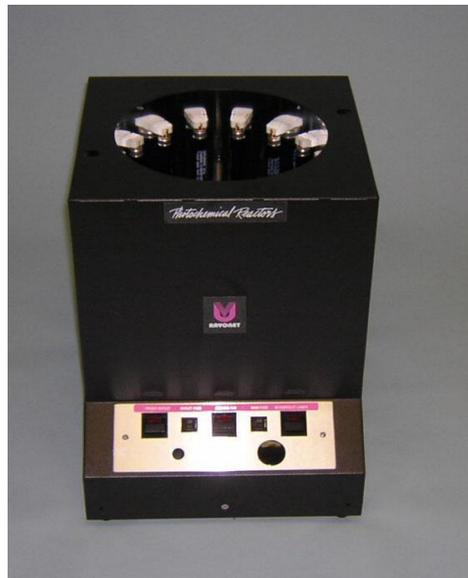
Figura III-4:Reactor Rayonet
